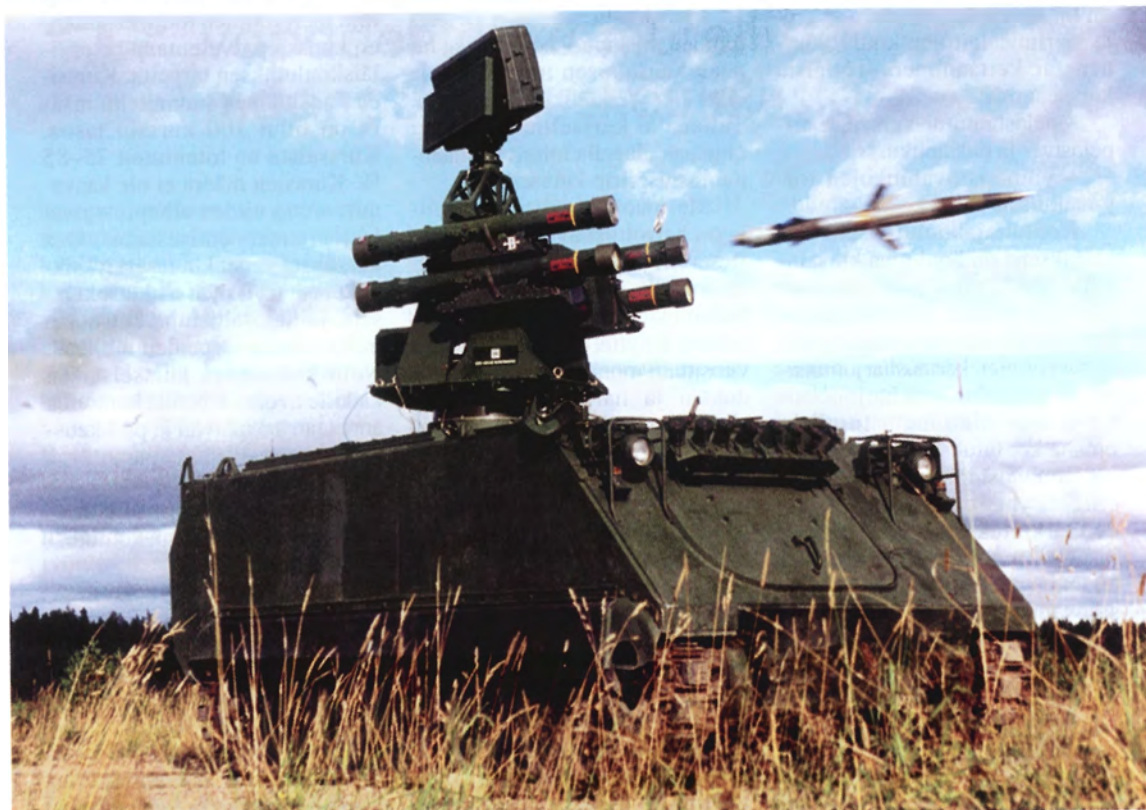
The ASRAD-R on the M113 chassis. The system can be installed on a range of tracked or wheeled carrier vehicles.
